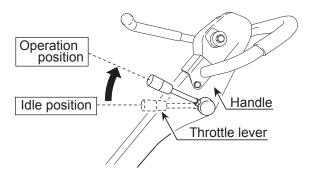
**Figure 16. Throttle Lever (Operation Position)**
